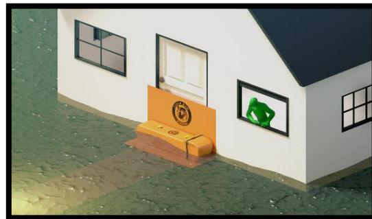
**Step 12:** Open both yellow valves and attach ½ inch garden hose attachment to garden hose. Fill water into either valve and close both valves once filling is complete. It's important to not overfill the tube. Do not fill the tube past the bottom of the top white pvc pipe.
